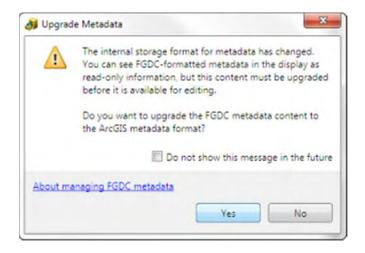
Click Yes to upgrade the existing FGDC metadata content right away. The Upgrade Metadata tool opens and the Upgrade Type is automatically set to FGDC\_TO\_ARCGIS.
