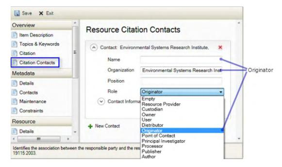
6. On the Contacts page under the Metadata heading, click New Contact if a contact doesn't already exist. Identify the point of contact for the item's metadata, including all relevant contact information. If an organization has been identified, this will be considered the primary contact when information is exported to an FGDC-format XML file.
