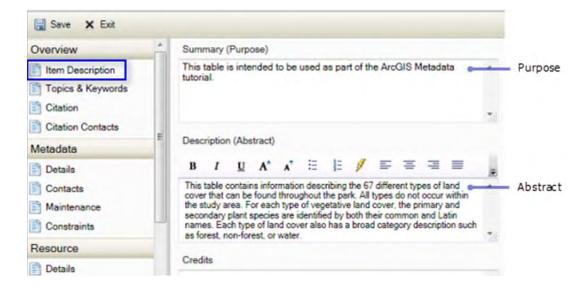
Use constraints may also be provided in the Use Limitation text box. If there are no use constraints associated with this item, leave the Use Limitation text box empty. The text None will be added automatically in the FGDC Use Constraints element when you export metadata to an FGDC-format XML file if use constraints haven't been provided.
